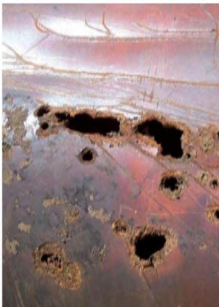
...pitting corrosion, induced by microbial metabolic products
