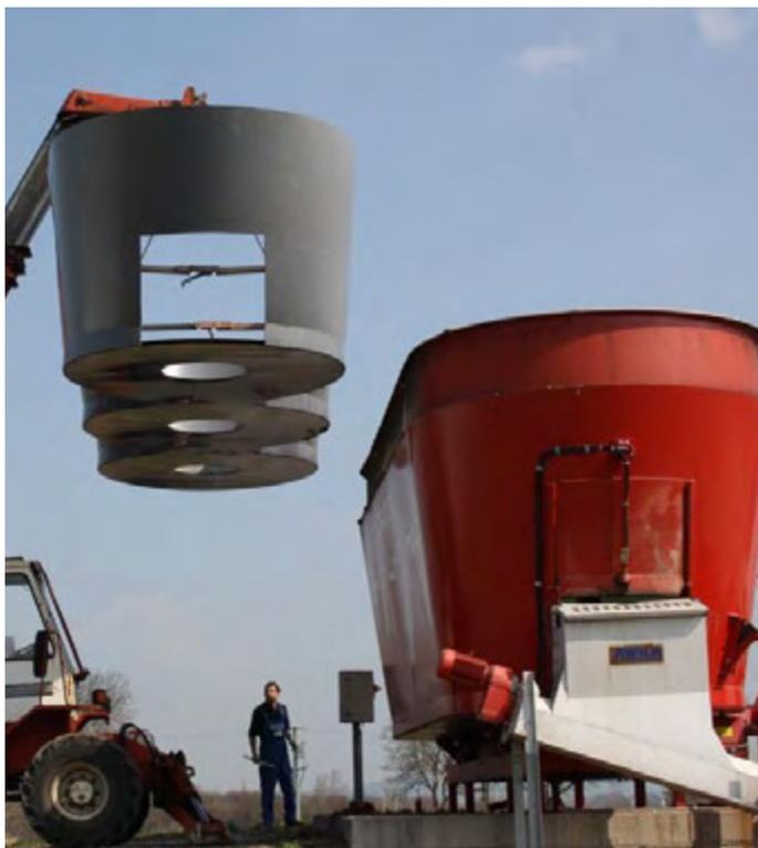
Due to the internal coating the substitution tanks are optimally protected against chemical attacks of herbal and animal substrates. The external coating prevents the tanks from general corrosion and abrasion effects.
