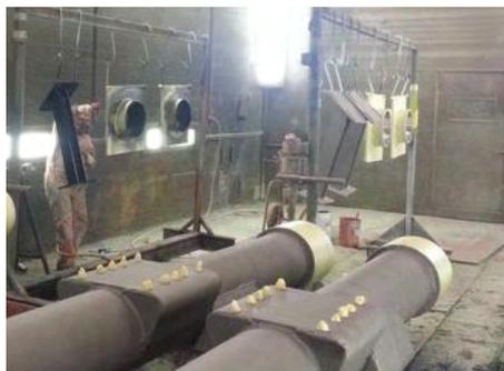
The shafts and pillar constructions were coated in one layer with our chemically resistant premium product PROGUARD CN 200 by airless spraying methods.
