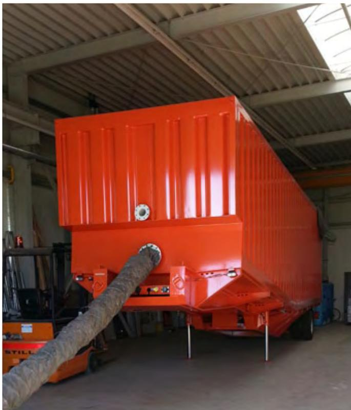
The trailer has a capacity of 79 cu. meters and is destined for the transport of 20% hydrochloric acid. There are very few coatings available, which show a sufficient resistance against such aggressive and highly corrosive liquids.
