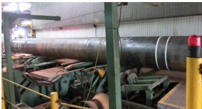
Internal coating of the intake risers
