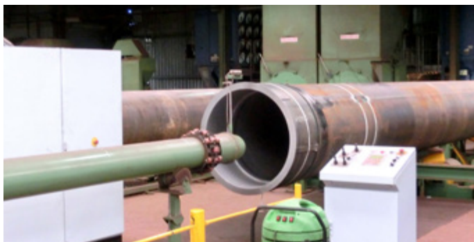
Internal coating of the intake risers
