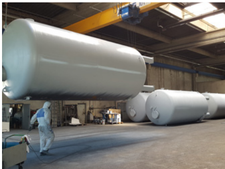
The external coating was carried out with a standard protection product.
