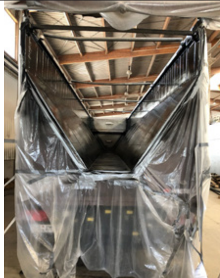
Finish: PROGUARD CN-1M is applied in two layers of 250 µm each.
