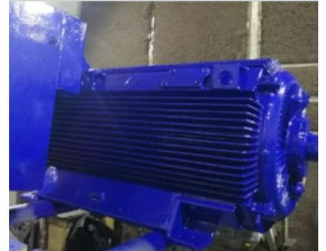
The top coat **PROGUARD 169(37)** was also applied on edges by brush, then sprayed wet-on-wet by airless in 2 layers with a total DFT of 80 µm.
