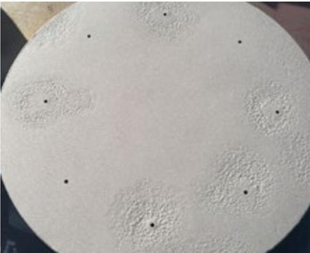
Prior to the coating the surfaces were cleaned with **803(E)**, afterwards sand blasted according to purity level SA3 and an average surface roughness of 75 µm.
