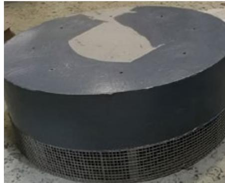
**ARC 858(E)**, a ceramic reinforced thick-film coating system especially for erosion-prone areas, was used for the smoothing and filling of the damaged surfaces. The curing time was 20 hours at 15 °C.
